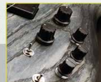
Ibanez 3-band EQ with EQ bypass switch & Mid frequency switch
