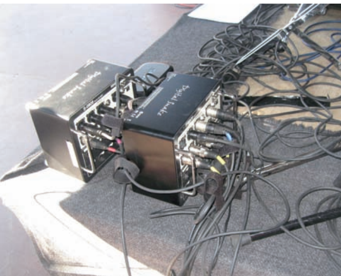
Klein, kompakt und REAC powered (REAC = Roland Ethernet Audio Communication) – die Roland S-0808 Digitalcores
